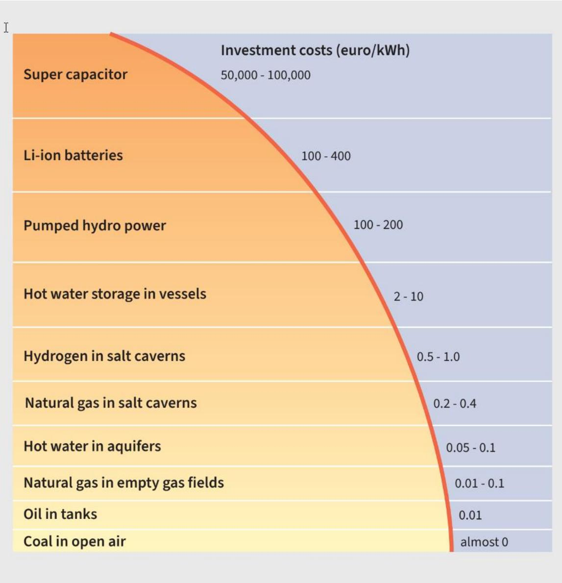
**Hydrogen storage in salt caverns is 100 to 200 times cheaper than electricity storage in pumped hydro power**
