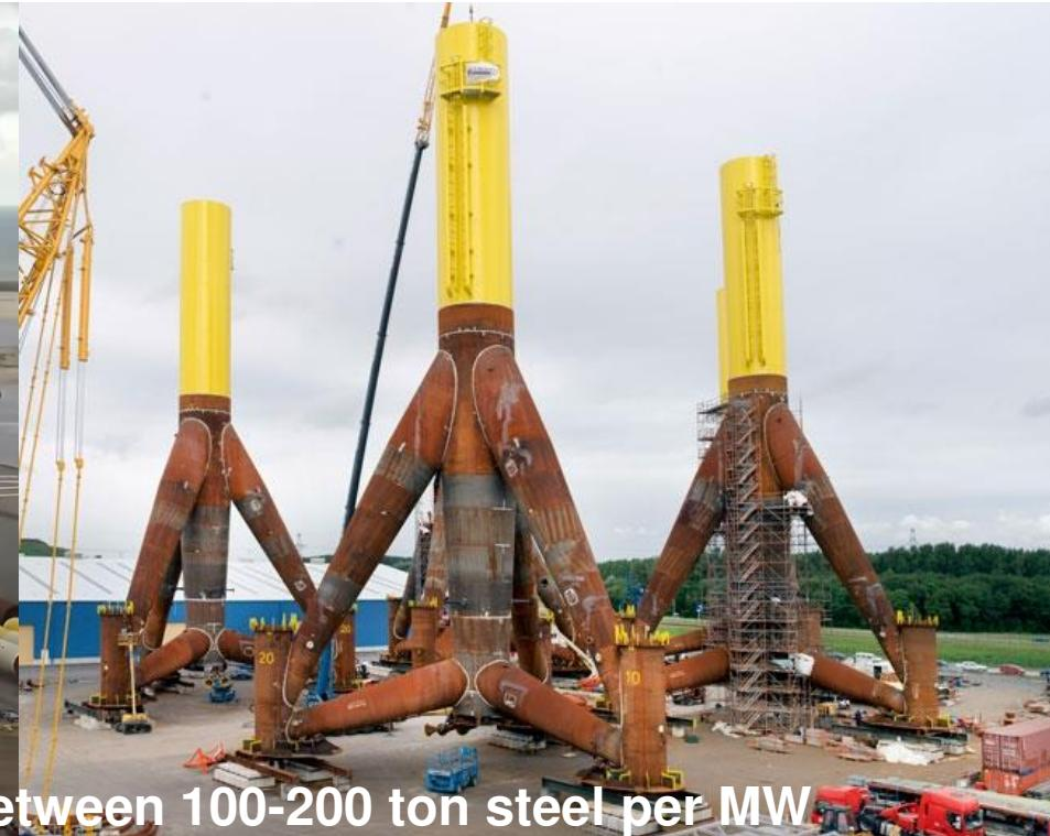
Offshore wind turbine require between 100-200 ton steel per MW
